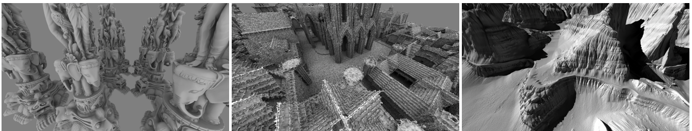
Figure 1: Thai Statues (200 M triangles), Displaced Rungholt (100 M triangles), and Landscape (132 M triangles) micro-poly geometries rendered with a diffuse path tracer at 1920 \times 1080 with > 20 fps (1 spp, denoising included). All micro-poly geometries are clustered and compressed prior to rendering. For each frame a LOD subset of clusters ( \sim 16 - 40 M triangles) are decompressed, converted and fused together into a BVH suitable for hardware-accelerated ray tracing. With a per-frame overhead of just 5.7 – 9 ms, our approach is suitable for real-time applications.
