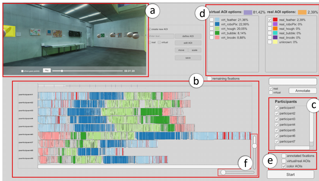
Figure 1: Overview of the presented visualization approach for the annotation of areas of interest (AOIs) in augmented reality. (a) A 3D gaze player and (b) a linked timeline view show fixations of participants on AOIs. The overview can be (f) zoomed and filtered for (c) participants and (d) AOI labels. (e) Different view options allow encoding annotated fixations differently to examine various aspects.
