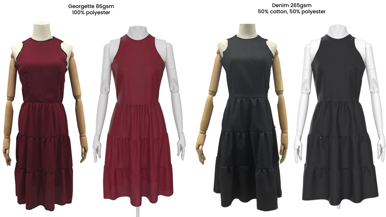
Figure 35: Comparisons of real garments on a mannequin, with virtual garments simulated using our engine and material model, for two different fabrics with different mechanical properties. On the left, we show a lightweight georgette, on the right, a thicker denim.
