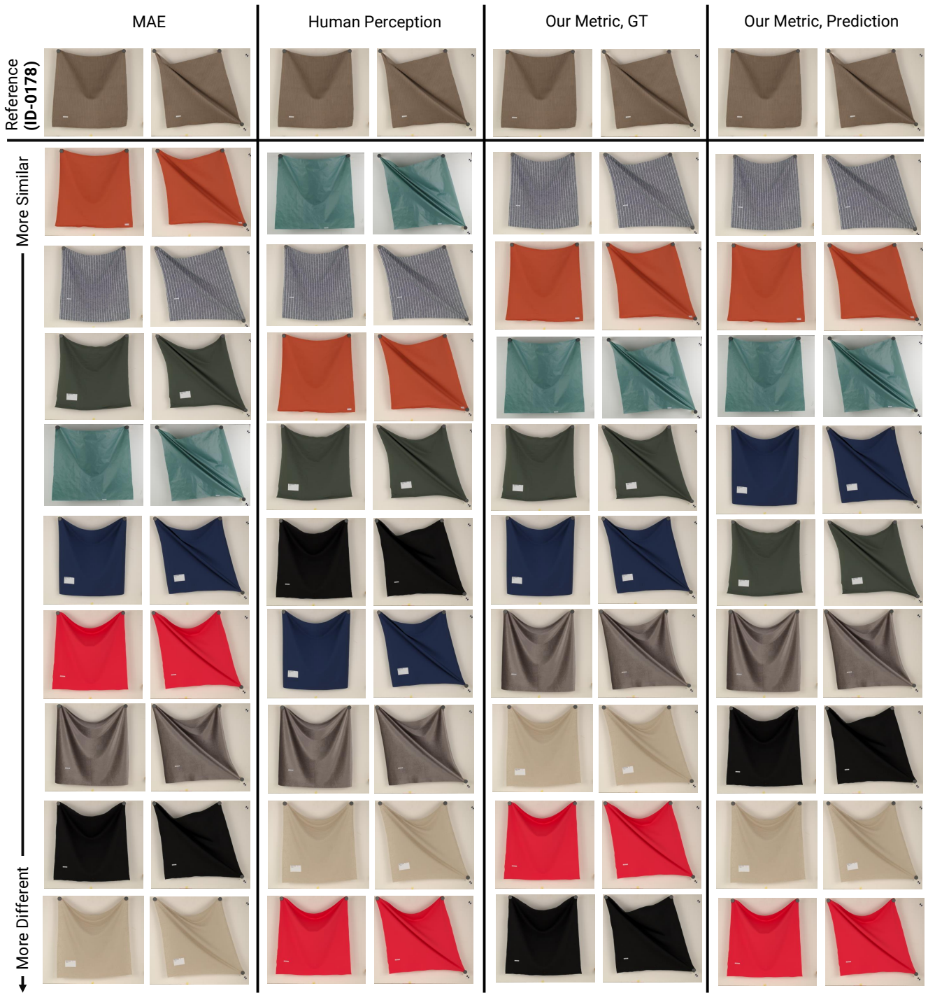
Figure 38: Relative orderings obtained for the fabric ID-0178 of our test set, using the similarities provided by comparing the materials on the parameter space (leftmost column), the tSTE embedding (center-left column), our Drapé Similarity Metric evaluated using the Ground Truth parameters (center-right column), and our Drapé Similarity Metric evaluated using the Ground Truth parameters (rightmost column).
