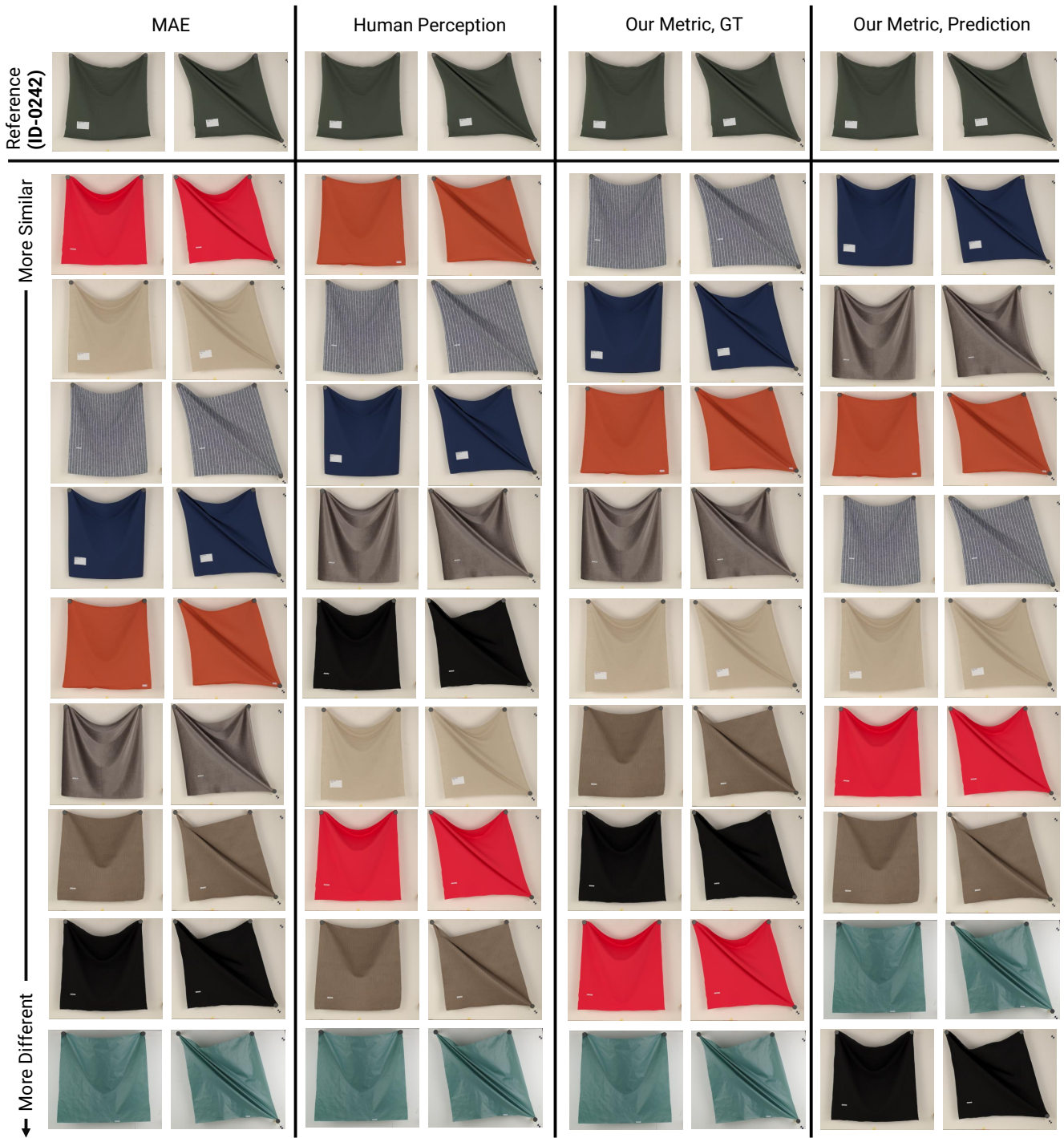
Figure 45: Relative orderings obtained for the fabric ID-0242 of our test set, using the similarities provided by comparing the materials on the parameter space (leftmost column), the tSTE embedding (center-left column), our Drape Similarity Metric evaluated using the Ground Truth parameters (center-right column), and our Drape Similarity Metric evaluated using the Ground Truth parameters (rightmost column).
