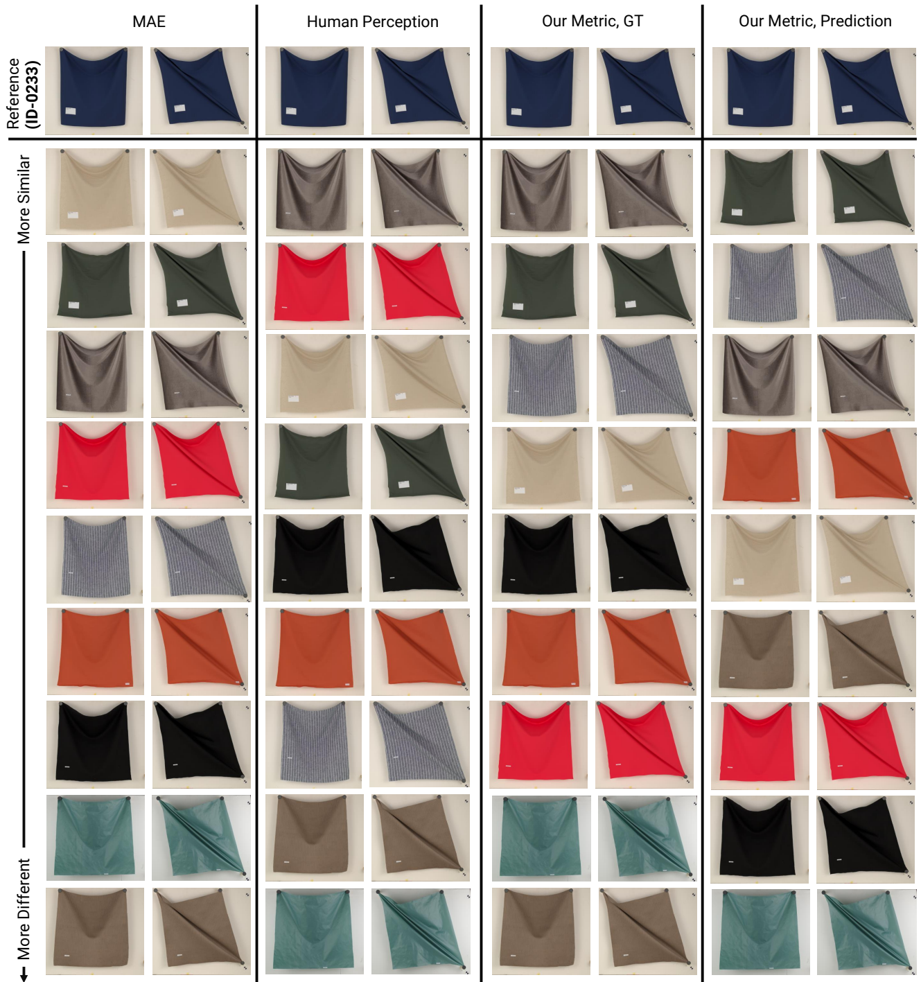
Figure 43: Relative orderings obtained for the fabric ID-0233 of our test set, using the similarities provided by comparing the materials on the parameter space (leftmost column), the tSTE embedding (center-left column), our Drape Similarity Metric evaluated using the Ground Truth parameters (center-right column), and our Drape Similarity Metric evaluated using the Ground Truth parameters (rightmost column).
