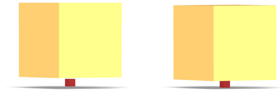
Figure 6: A heavy rigid block (yellow) is dropped on a much lighter block (red) where it then comes to rest. The mass ratio between the blocks is 1000 : 1. Our contact handling method is able to robustly handle this challenging constellation.
