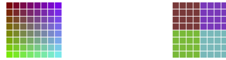
Figure 3: Two examples of best possible 2D arrangements for 64 colour samples. Left: The perfect HD (3D) order is preserved. Right: Four different colours with 16 samples each, here the HD order cannot be preserved. Colours adjacent to a different colour on the 2D grid are not near their nearest HD neighbours.
