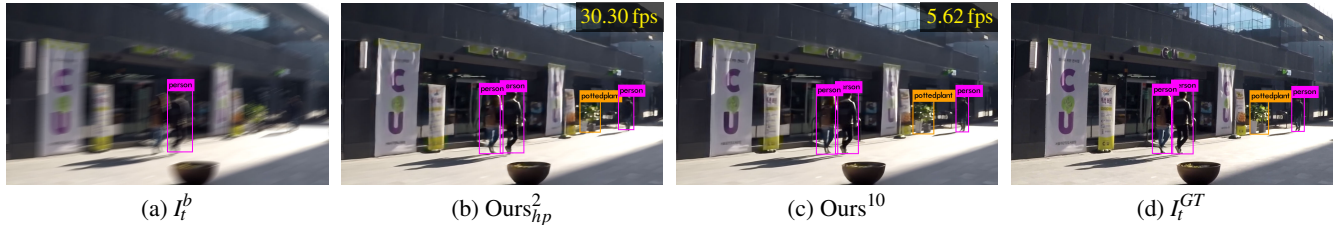
Figure 2: Object detection results. Deblurred results of our (a) 2-stack and (b) 10-stack models improve the performance of the object detection task. Our real-time 2-stack model shows a comparable detection quality to that of the 10-stack model and can be useful when real-time processing is required (e.g., object detection for autonomous driving).
