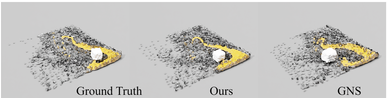
Figure 8: Ground truth vs. Our method vs. GNS for test scene without obstacle. The scene is not used for training. On average, our method yields less error, train and inference substantially faster than GNS and consume much less memory.
