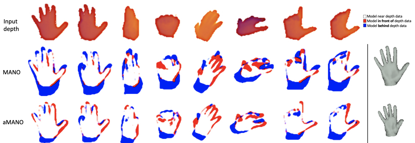
Figure 1: We introduce a new hand model, aMANO, by augmenting MANO's shape space with a local scale adaptation which enables calibrating to users with substantially different hand sizes than those covered by MANO. We also present a framework to calibrate and track aMANO by registering it to a sequence of depth frames. Here we see that aMANO registers more accurately than MANO for a child's hand sequence. We show the calibrated mesh in the rest pose for MANO and aMANO in the rightmost column.
