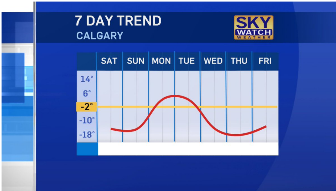
Figure 5: Stage: Perception Category: Visual Illusion Tag: Inappropriate Use of Smoothing Tag Description: Line smoothing techniques cause interpolation between data points and can even create non-existent data points. Visualization Description: The seven-day trend chart above indicates that the highest temperature is reached at midnight between Monday and Tuesday, which is completely incorrect.
