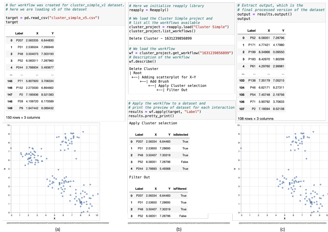
Figure 6: Executing a computational workflow defined in the visualization tool in a computational environment. (a) We first load the dataset. (b) We load the workflow library and the workflow we are interested in. We then apply the workflow to the dataset. The tool plots a preview of the actions. Note that new isSelected and isFiltered Boolean column are introduced when a brush and filter are added in the preview. (c) After the filter is applied, the number of rows is reduced from 150 to 108. A visualization of the result shows the cluster was removed. Visit the notebook .
