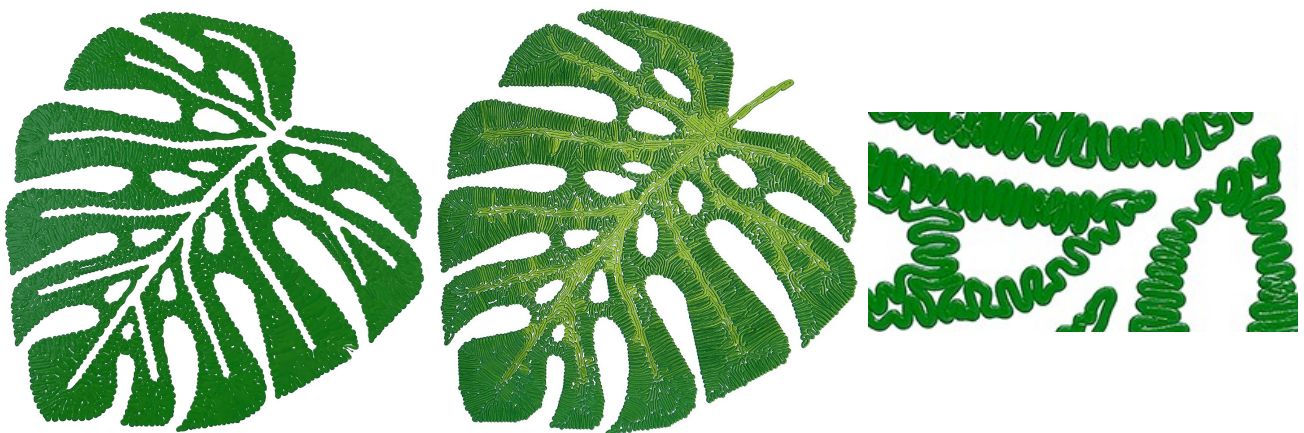
Figure 18: Left: Single material leaf printed with a constant width smaller than nominal to appreciate the cycle folds. Note how the cycle goes around holes with a single folded trajectory in the center part. Middle: Multi-material version using a narrower spacing, with the inner skeleton in a different material. Right: Closeup. Note how the cycle locally has a single trajectory around the holes. Such cycles cannot be obtained by growing from a small circle to invade the surface: this always gives an even number of paths in between outer contours.
