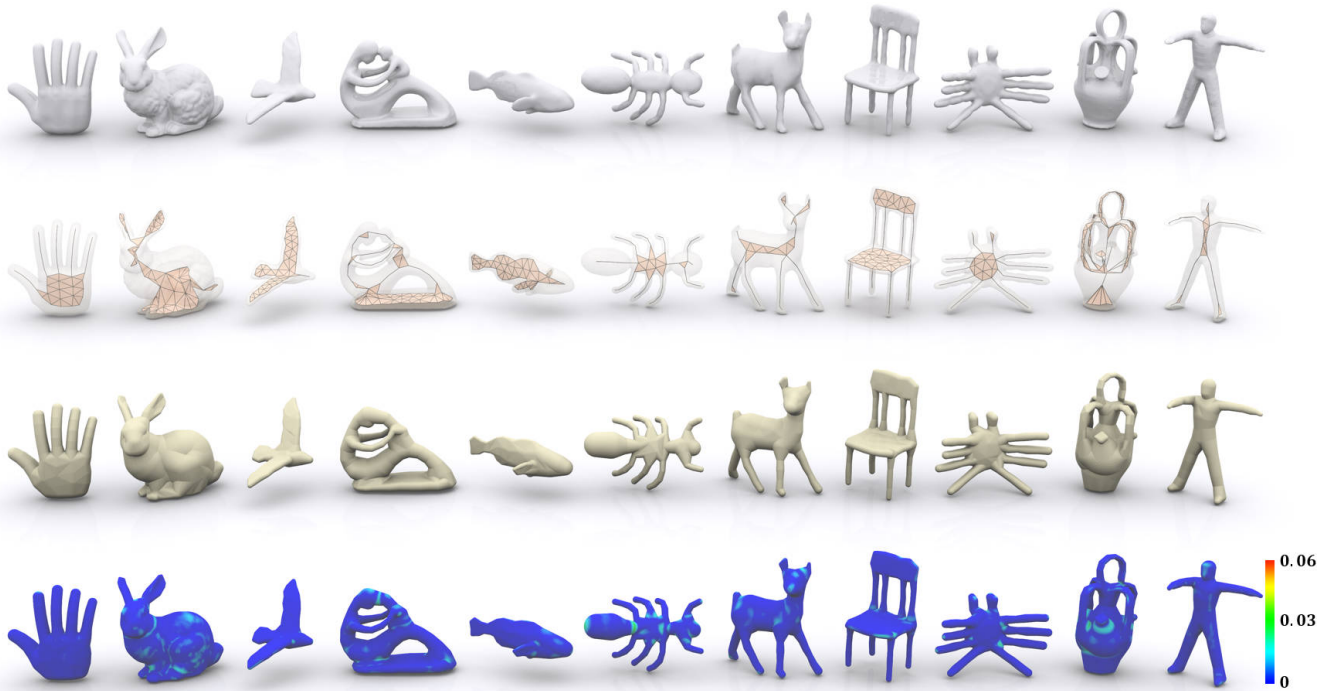
Figure 4: Shape approximation results of Coverage Axis. First row: the input shapes. Second row: the output skeletal representations for MAT approximation. Third row: the reconstructed shapes by the skeletal representations. Fourth row: color coding of the reconstruction error between each point in the reconstruction and the input shape, defined relative to the diagonal length of the bounding box.
