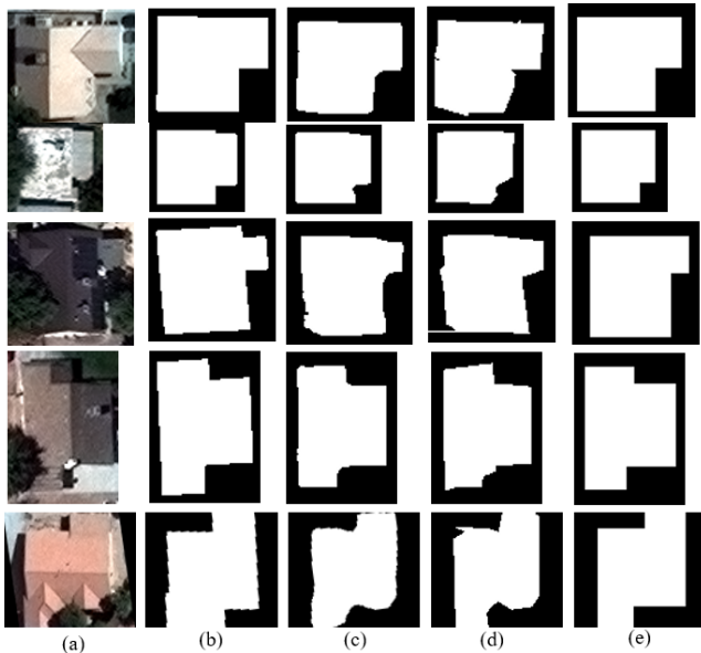
Figure 10: Qualitative Comparison. (a) Real images. (b) Ground truth footprints. (c) Initial building footprint segmentations. (d) ASIP results. (e) Our results.
