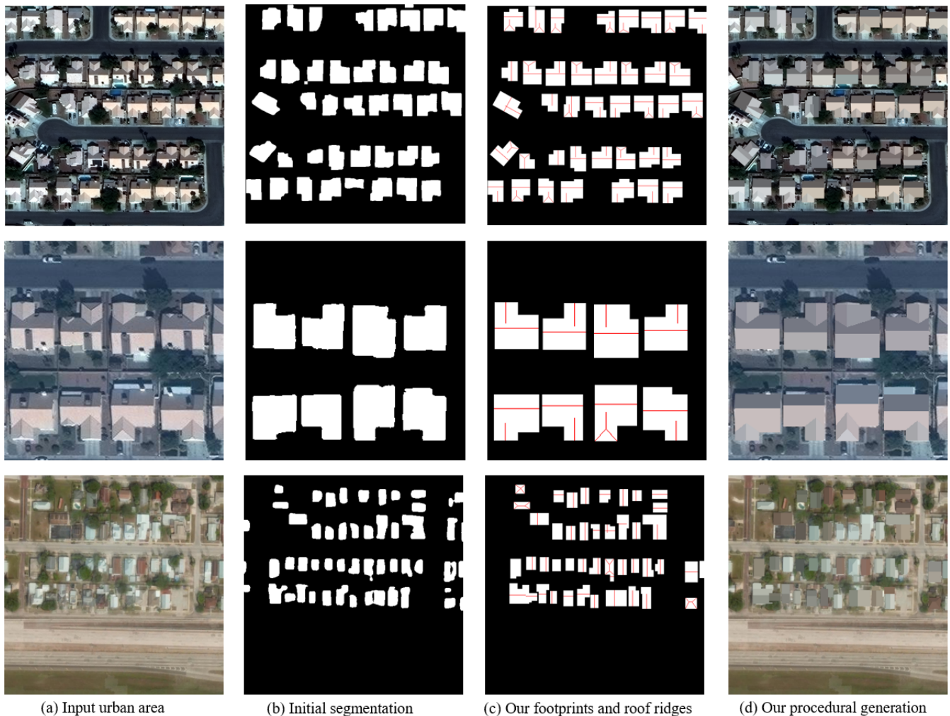
Figure 13: More examples. (a) Input urban areas from SpaceNet, CrowdAI and Urban3D respectively. (b) The initial segmentation of (a). (c) Our decomposed roof parts and predicted ridges. (d) Our procedural outputs on top of real image (a).
