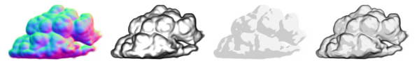
Figure 7: The differentiable sketcher computes normals, contours, and toon shading (from left to right), and combines them into the final sketch (right).
