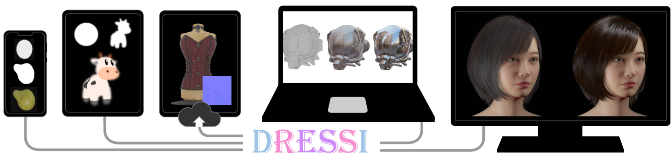
Figure 1: Applications of our differentiable renderer called Dressi. From left to right: optimization of geometry and material (a pear and a cow), normal map, environment map and material, and hair material of the digital human. The applications work on all devices supporting a modern graphics API Vulkan [Khr21] such as mobiles, tablets, cloud servers, laptops, and desktop PCs.
