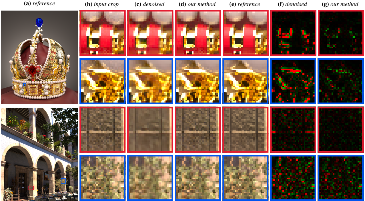
Figure 9: Visual comparison of our trained models (HDR, ALB, NRM, VAR of Table 1): denoising (c,f) versus our method (d,g). In the difference images (f,g), negative difference is red, positive is green, and values are uniformly scaled for visual clarity. RMSE of the denoised and progressively denoised images are 0.139 and 0.043, respectively, for the top scene (1024spp input), and 0.028 and 0.018 for the bottom scene (256spp input).
