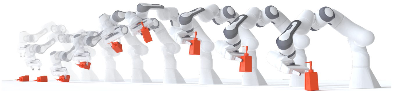
Figure 1: Grasp and place the object to its upright orientation guided by our UprightRL model.
