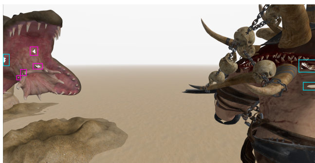
(a) On the borders of the screen, the effect of premature frustum culling can be observed during animations of GIANT WORM and BUTCHER (cyan rectangles). Inside the GIANT WORM's mouth, some meshlets are prematurely backface-culled as a result of disregarding how the normals of triangles assigned to meshlets change through animation (marked in magenta).
