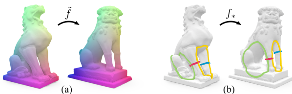
Figure 8: (a): A functional map \tilde{f} represented by 50 \times 50 coefficients. (b): The homology map f_* obtained from \tilde{f} by our inference.
