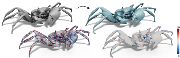
Figure 21: We use our normal driven editing to deform the input shape (gray) into a piece-wise developable approximation (blue). In the bottom row, we visualize the Gaussian curvature concentrates on the creases after the deformation, leading to a piece-wise developable shape. ©Oliver Laric under CC BY-NC-SA.
