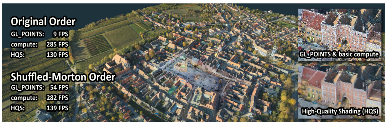
Figure 1: Performance of GL_POINTS compared to a compute shader that performs local reduction and early-z testing, and a high-quality compute shader that blends overlapping points. Retz point cloud (145 million points) courtesy of Riegl.
