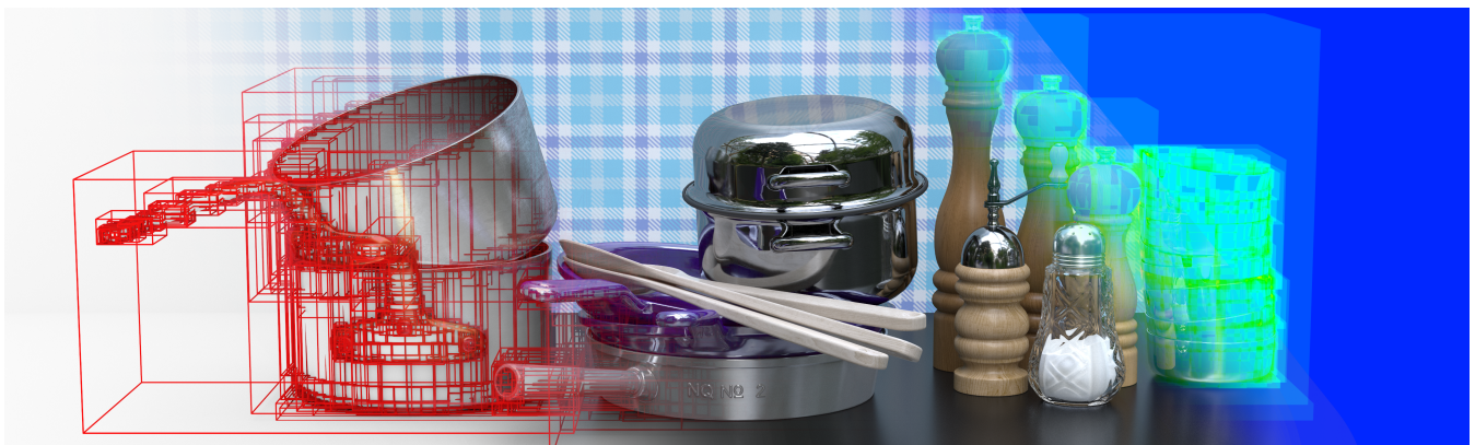
Figure 1: Bounding volume hierarchies (BVHs) are the ray tracing acceleration data structure of choice in many state of the art rendering applications. The figure shows a ray-traced scene, with a visualization of the otherwise hidden structure of the BVH (left), and a visualization of the success of the BVH in reducing ray intersection operations (right).
