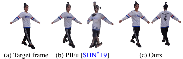
Figure 11: Comparison with a learning-based method. Textures for the target frame (a) are reconstructed by PIFu (b) and our method (c). In PIFu, the input is a single RGB image with low resolution. The reconstructed textures are blurry (b left) for the visible regions in the input, and contain artifacts (b right) for the invisible regions.
