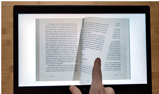
Figure 10: The user controls the active page by moving their finger on the screen. The page follows the thus-defined positional target while behaving like a real paper surface.
