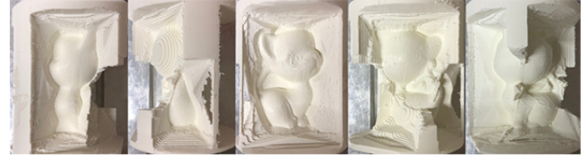
Figure 16: Finishing phase. Side regions finished with a Imm ball cutter.
