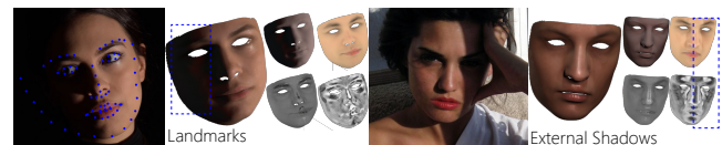
Figure 10: Limitations – left: Imprecise landmarks under extreme scene illumination produces incorrect geometry reconstruction. Right: External shadows get baked into albedos.
