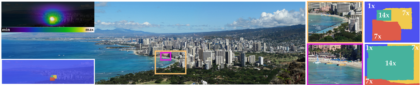
Figure 12: Honolulu: The 14x effective zoom gives the 108MP collection an implied resolution of 9.1GP. All images were captured in 2 min. Inset are two interesting detailed portions (orange, purple) of the image along with their graph cuts segmentations. In addition, the full seam segmentation along with the navigation field are provided.
