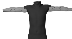
Figure 11: The body is segmented into three overlapping parts (left arm, right arm, and torso). The vertices selected for collision detection are shown as light gray dots.
