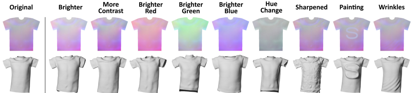
Figure 2: Various image editing operations applied to a given cloth image (top row) and their corresponding modified cloth shapes (bottom row). Note that although the wrinkle lines blended into the image in the last column are hard to see, the resulting wrinkles are clearly visible.
