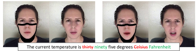
Figure 13: Text-based Editing of Talking-head Video [FTZ*19]. An editor changes the text transcript to create a new video in which the subject appears to be saying the new phrase. In each pair, left: composites containing real pixels, rendered pixels and transition regions (in black); right: photo-realistic neural-rendering results. Images taken from Fried et al. [FTZ*19].
