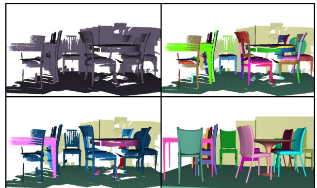
Figure 14: Data-driven object reconstruction. The search-classify approach [NXS12] initially over-segments the scene (top-right) and search-classifies meaningful objects in the scene (bottom-left); these are reconstructed by templates (bottom-right) overcoming the high clutter present in the input scans (top-left). Source images courtesy of Nan et al. [NXS12].
