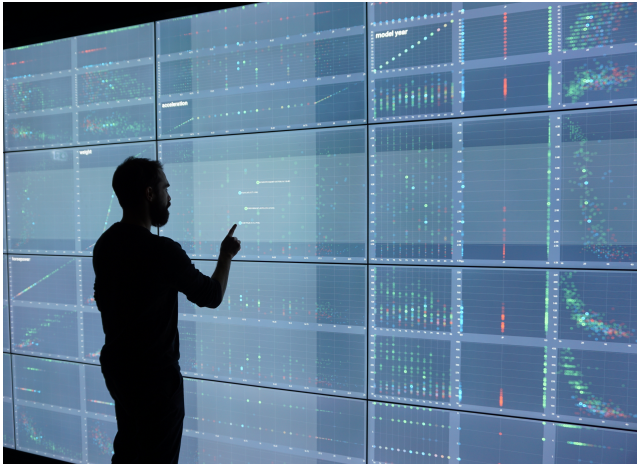
Figure 1: Touch-enabled visual analysis using SPLOMs on a large wall display ( 4.08 \times 2.31 m). Our two-tiered Focus and Context (F+C) technique with an outer F+C at matrix level and an inner F+C within scatterplots improves the exploration process by giving access to detail even in dense areas (see Subsection 3.1).
