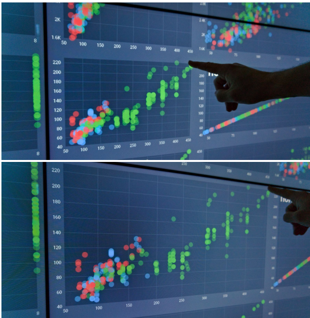
Figure 4: Global F+C by directly resizing a plot. (top) The user long-taps on the corner of the plot to initiate a horizontal and vertical resize. (bottom) The plot corner moves along with the finger and therefore the plot expands. The plots to the right and top shrink accordingly.
