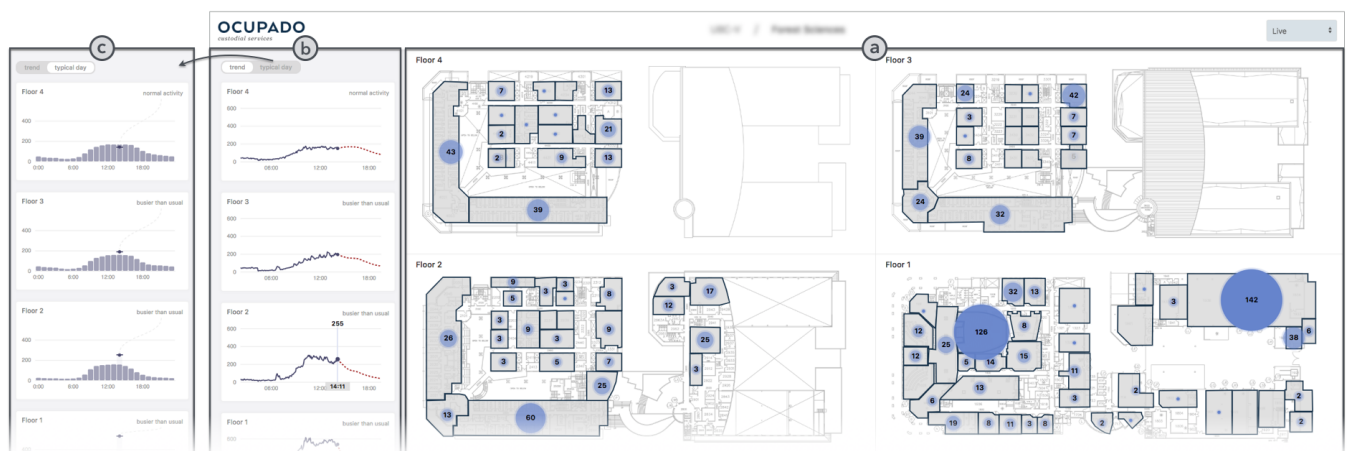
Figure 1: Building Recent Interface, overview window. (a) Floor plans sized to all fit within one screen with zone-level superimposed circle symbols showing live device counts. (b) Per-floor aggregate trend charts showing device counts over past 12 hours and prediction for the next 3 hours (red dashed line). (c) Alternative sidebar showing aggregate per-floor usage for typical day vs. current live data.
