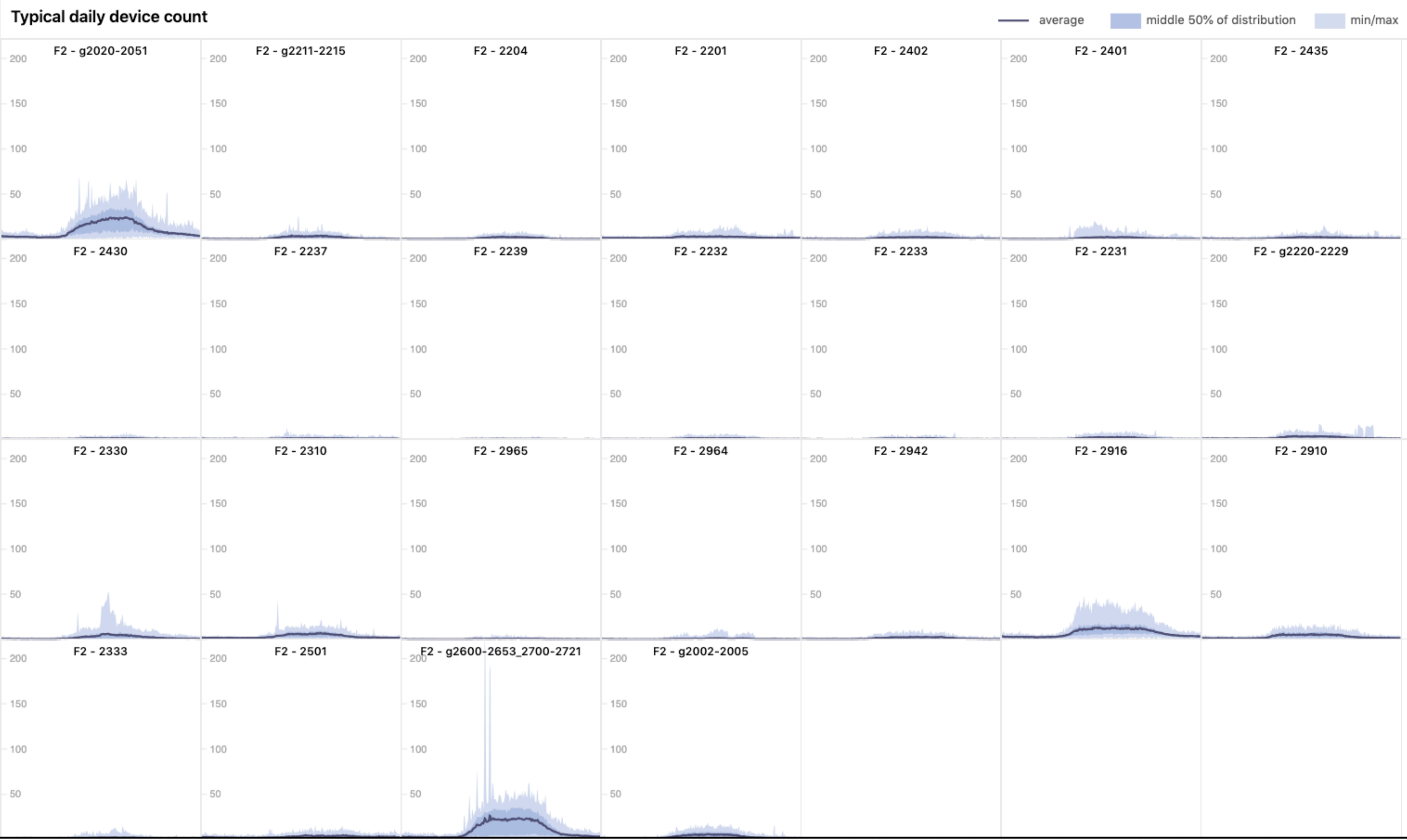
Building Long-Term Interface. Typical day profiles for many zones, automatically sized to fit onscreen. ZF-All:LA
