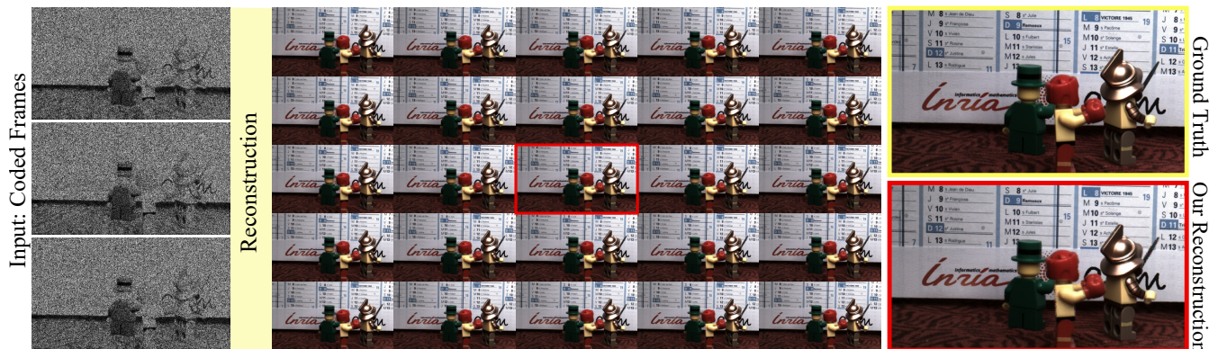
Figure 1: Reconstruction of a 6D light field video (middle) from 2D sensor images (left). Each 2D image contains samples from angular and spectral dimensions convolved with a random color-coded mask that changes per-frame. The proposed algorithm reconstructs the full resolution color light field video using a novel sensing model, together with a temporally-aware learned dictionary. On the bottom right, the magnified image of one angle of the reconstructed frame is shown with the corresponding ground truth on top.
