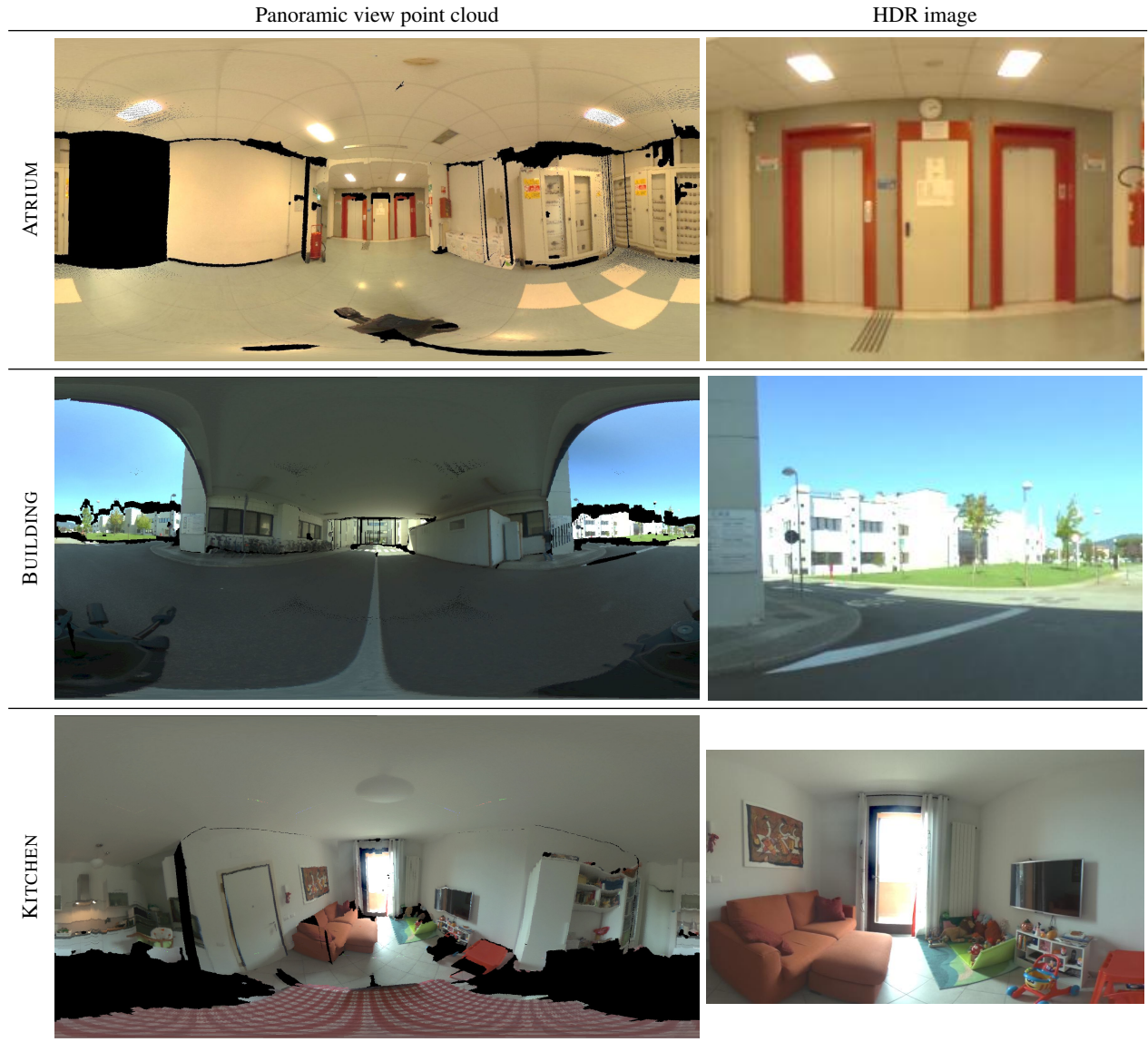
Figure 2: Input dataset with an equirectangular view of the point cloud and the input HDR image used for the expansion. These dataset have a ground truth HDR color for each point of the cloud. The point clouds were reconstructed from a single HDR panoramic image with a user-assisted method [BCD* 13].
